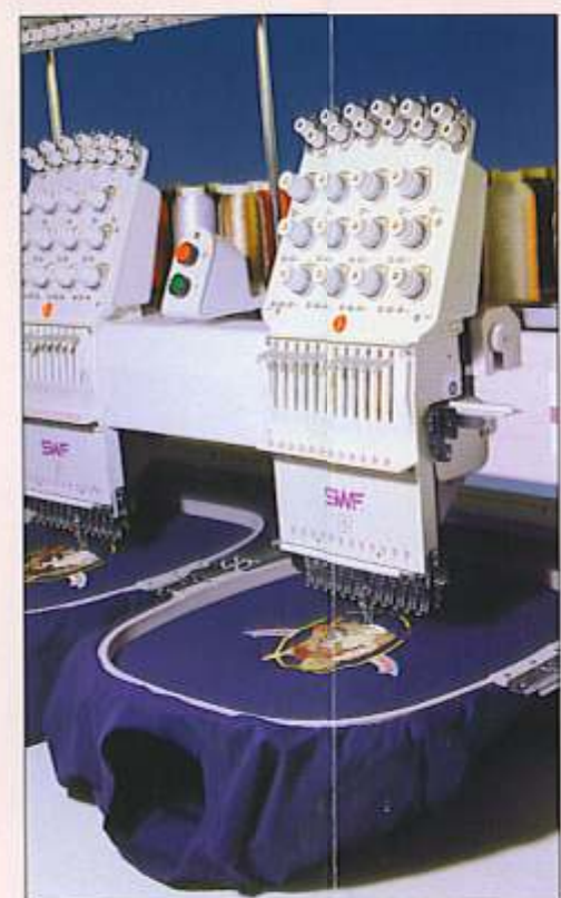
▲ Tubular Frame Work The wide embroidery range of 419mm(X) x 439mm(Y) at the maximum enables us to handle the large size of tubular materials.
