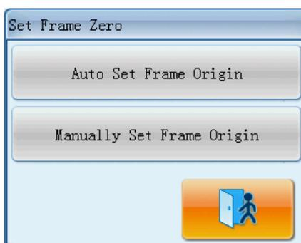
Select “Auto Frame Origin” and then click “Confirm”. At this moment, the frame will automatically find the origin and confirm it. (**Note:** when the limits coupler is damaged, user can use “Manual Frame Origin” to confirm the frame origin.)
