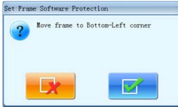
Use the move frame key on panel to move the embroidery frame, confirm down-left corner point of soft limit position and click
