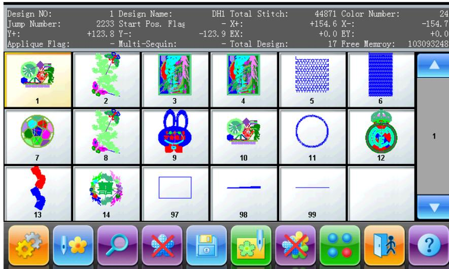
In “Other Design Management Functions”, click “Edit Design” key, after which, in the activated dialog window, click to start editing the current design; Click “Create New Design” to edits a new design; the detailed operations of “Edit Sequin of Current Design” will be explained in the chapter of JF Type sequin embroidery operations. (Note: the design selected can not be combined design, or system will give the warning of “not common design”)
