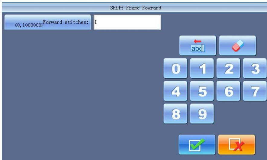
4. System returns to the main interface, press
