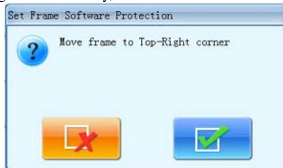
Use the move frame key on panel to move the embroidery frame, confirm the upper-right corner point of soft limit position and click
