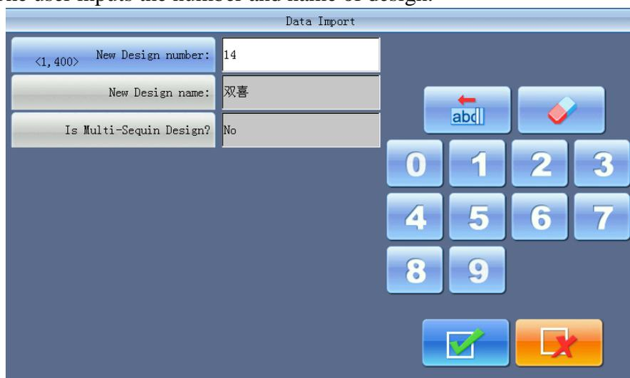
The system provides the minimum available design number as the default value. The customer can use the small panel to change the value. Refer to sequin operation for “Is multi-sequin Design?”. When several designs are input for one time, the user can only input the number for the first design.
