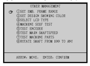
3. Press "2" to select "SELECT DESIGN SHOWING COLOR" and then press "-" to enter the color adjusting screen.
